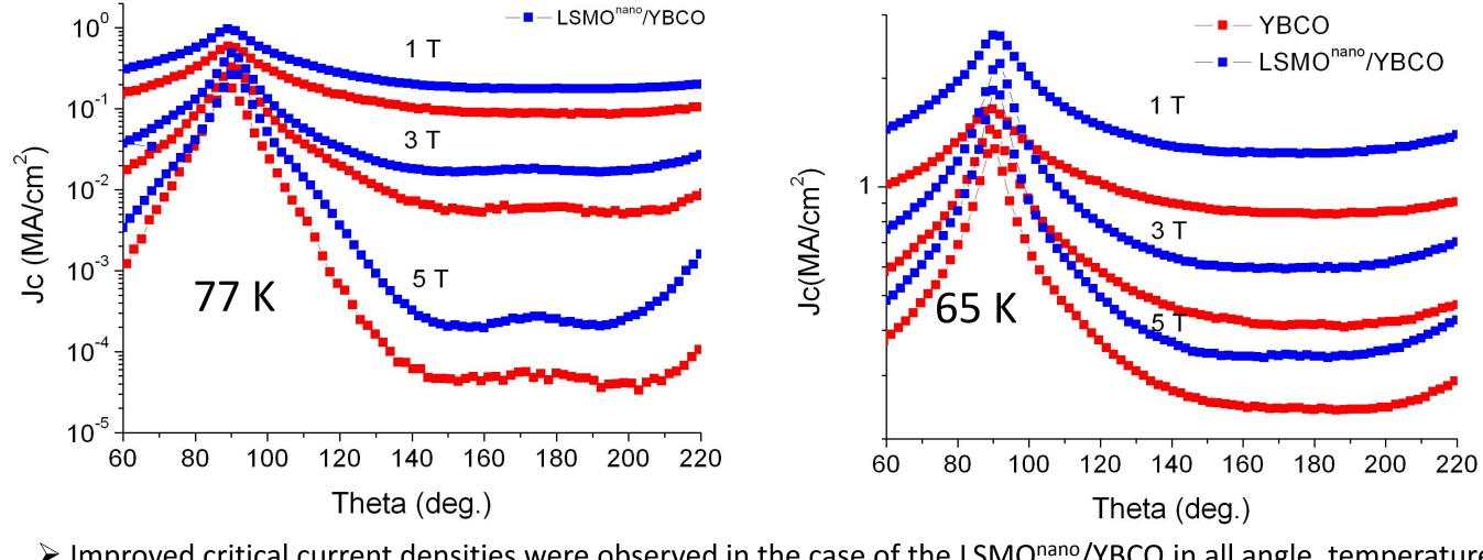
> Improved critical current densities were observed in the case of the LSMO<sup>nano</sup>/YBCO in all angle, temperature and field ranges;
