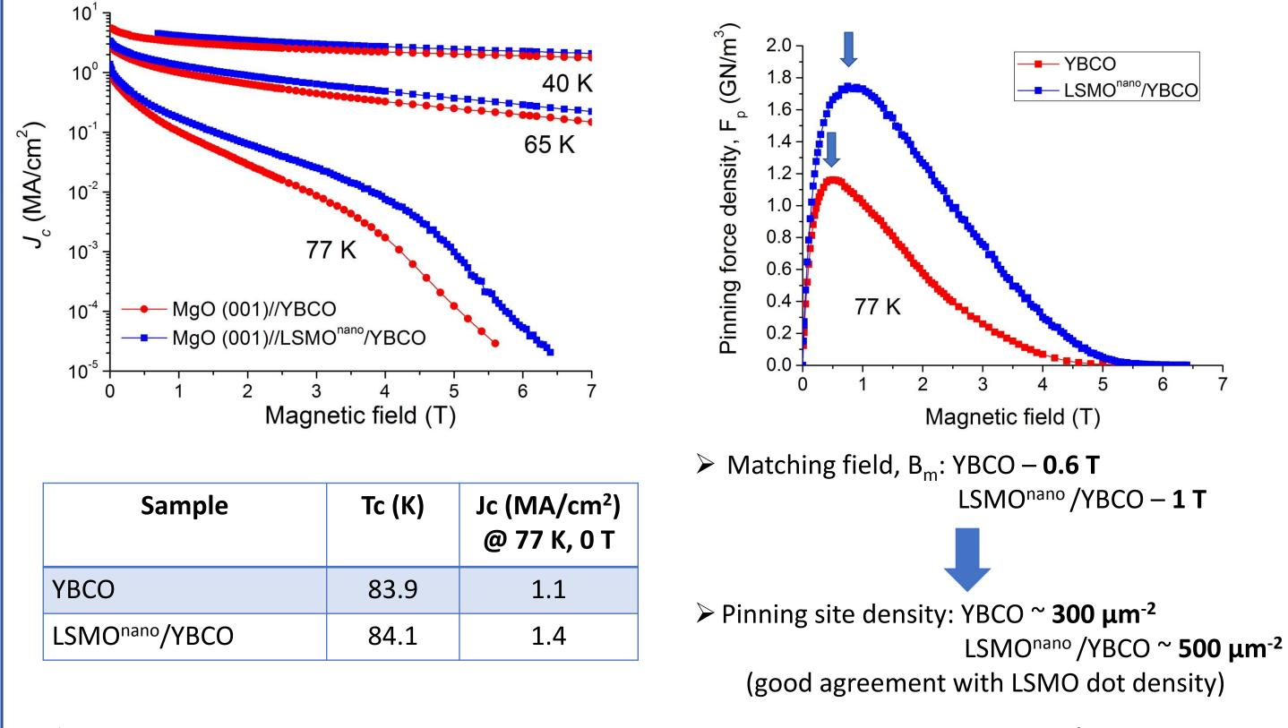
> Superior current carrying capabilities were demonstrated in the case of the LSMO<sup>nano</sup>/YBCO film over the whole magnetic field range at different temperatures
