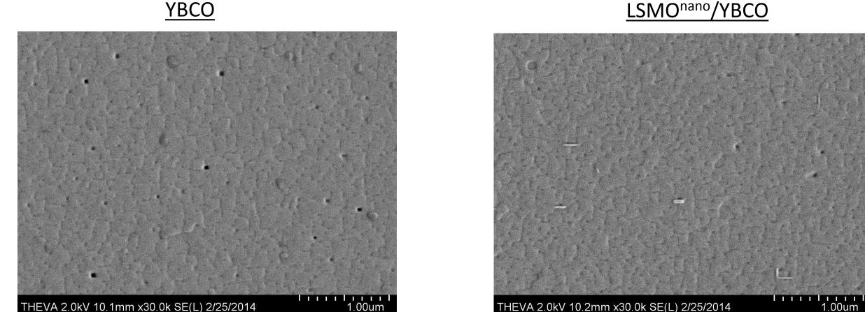
> YBCO 100 nm thick films were deposited by co-evaporation technique (ceraco GmbH) good homogeneity, very low rms roughness, 2-3 nm (evaluated by AFM) > smaller grain size in the case of the YBCO film grown on decorated substrates
