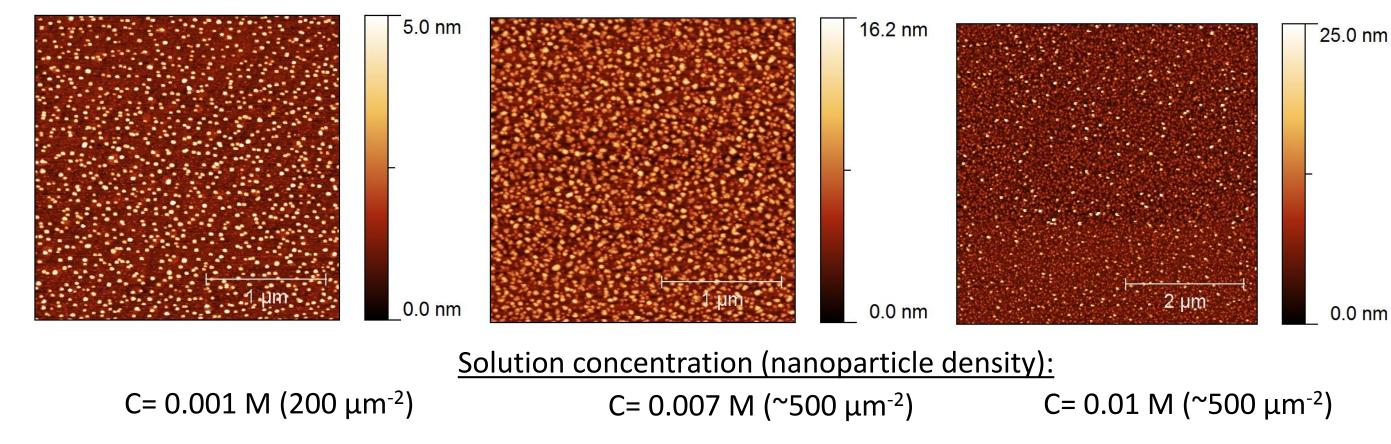
$\blacktriangleright$  Nanostructure densities appear to saturate above C = 0.005 M to approximately 500  $\mu$ m<sup>-2</sup>;
